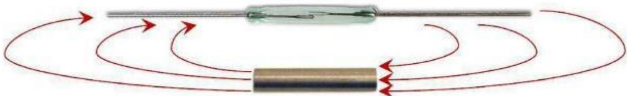
Figure 2 – Magnetic Flux
