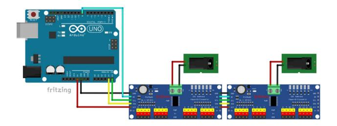
It should be noted that the supply of the individual servos can no longer be taken from Arduino here at the latest, but that it is imperative that the supply voltage is externally supplied via the green terminals. One external power supply per module must be supplied.
