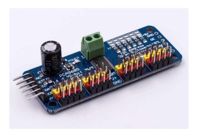
The PCA9685 module is an I2C bus controlled 16 channel PWM controller module for Arduino and Raspberry Pi applications with servo motors. Each PWM servo output has a separate internal PWM controller with 12 bit resolution (4096 steps).
