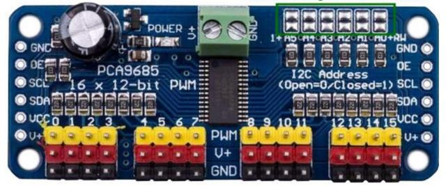
The addressing solder bridges A0 to A5 on the module should then be connected differently for each module according to the binary code counting upwards:
