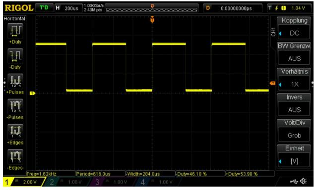
Max. PWM base frequency with a prescaler value of 0x03h. (Here due to oscillator inaccuracy: 1.62 Khz)
