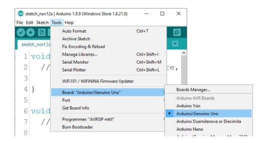
The port to which the Arduino board is connected has to be selected. Go to: Tools > Port > {port name goes here}
