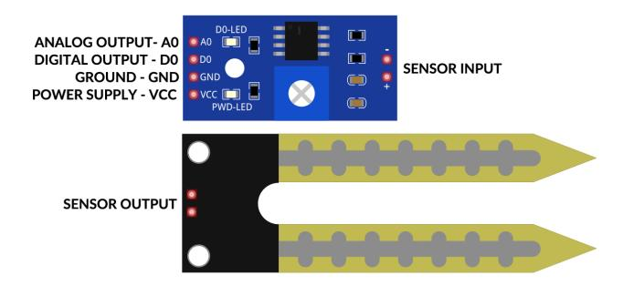
The sensor board does not have polarity, which means that two pins from the sensor board can be connected either way, on the control board SENSOR INPUT pins.
