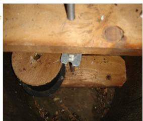
Place the motor on the piece of wood that you are using as a shelf. Move the motor as close as you can to the wall of the barrel with out any part of the motor touching the wall then screw the motor into the wood using some wood screws. Also go ahead and drill a hole in the back of the container for the plug to come out of.
