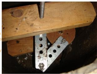
Take the second piece of wood that has the drilled hole in it and slide it on the rod 6 inches down from the top of the barrel. Secure in place with some screws. This will support the top half of the threaded rod.
