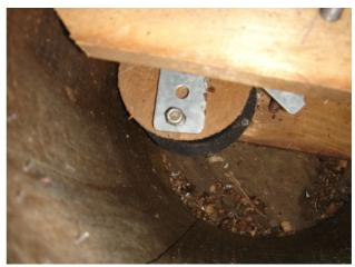
Next take the 2 foot threaded rod and screw a nut on the it about 8 inches in from one side. Take the other piece of flat bar and slide it on to the rod. Take another nut and screw that on top of the flat bar. Now there should be a nut on each side of the flat bar and do not tighten the nuts up against the flat bar yet. This is because we have not put in the motor yet and this flat bar needs to line up with the motor.
