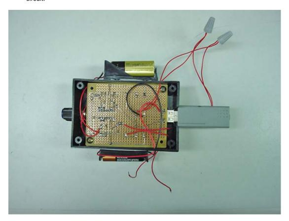
Caution: When installing the 9 volt battery, do not reverse the polarity, not even for an instant. This circuit is not fused, and reverse polarity will blow a crater (literally) in the 556 timer IC. I know I'm repeating myself, but the chip will explode. See for yourself:
