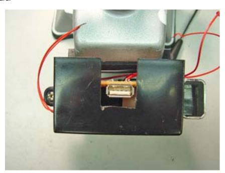
10. Here's where I soldered the player trigger wires. Make sure you don't get any solder on the other components or terminals. File a notch in the cover to let the wires out.
