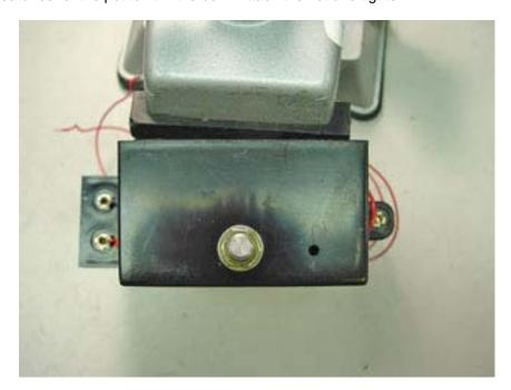
8. Again, I used foam tape to attach the AAA battery holder to the box. Solder the battery leads as shown in Step 4.
