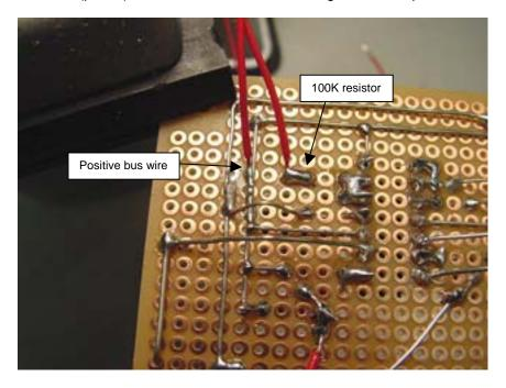
4. Solder the AAA battery holder to the remaining normally open pin on the DPDT relay and the pin shown on the USB connector. Note: If you plan to place this circuit in a project box, you may want to wait until the box is ready and the wire holes are drilled before making this connection.
