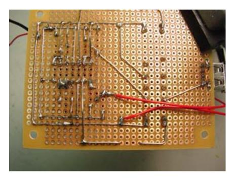
2. Solder two wires to the SPST relay as shown. These wires will connect to the MP3 player switch wires. Make them about 6"-8".
