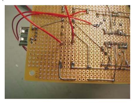
3. Solder two 6" wires as shown. These will connect to the 1Mohm potentiometer. The 100K resistor (pin 13) is the one that's next to the large 220 uF cap.
