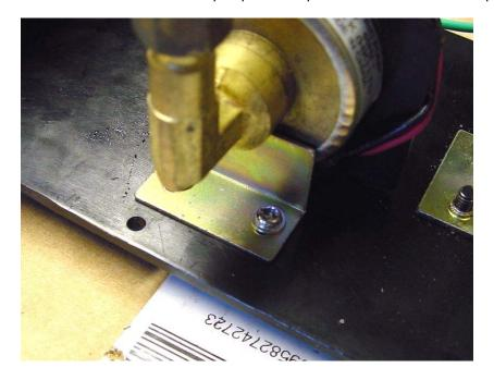
3. Remove the 2 screws that hold the pump bracket. Lift the bracket out of the bottom panel. The pump body can be pressed out of the bracket.
