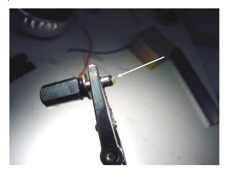
7. The reason my pump failed was that the end loop of the internal spring broke off, and the cap/O-ring fell out of the plunger. This can be fixed easily.
