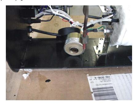
5. Lift the tube out of the elbow fitting. Rotate the elbow to remove it from the pump body. Caution: Depending on the nature of the pump failure, there may be small parts inside the elbow fitting. Look carefully to be sure that no parts fall out and get lost. There is a spring inside of the plunger. This spring may be able to fall out of the plunger. If it does, then this is your problem.
