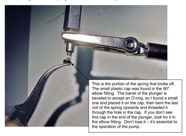
8. It's a bit difficult to get the O-ring on the cap, but keep trying and you'll get it. Use a tweezers to bend the last loop of the spring upwards as shown. Insert the spring into the plunger so that the spring loop can be hooked with a wire. Pull it out of the plunger as shown below and insert the loop through the hole in cap.
