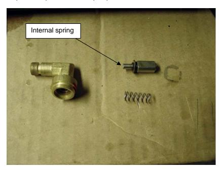
6. Your plunger should look something like this. If the cap on the end of the plunger is missing, look inside the elbow fitting. It may look like a bit of dried fog fluid. Do not lose this part!
