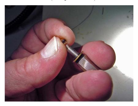
9. Now you have a repaired plunger. Check the other parts for debris, clogs etc before reassembling the pump. Inside the elbow fitting is a check valve. It is pressed into the fitting and can't be removed. Press carefully on the valve plate (at the bottom of the fitting) with a stiff wire to make sure that it depresses and returns easily. This valve is what allows the fluid to go into the heater and prevents vaporized fog from coming back into the pump.
