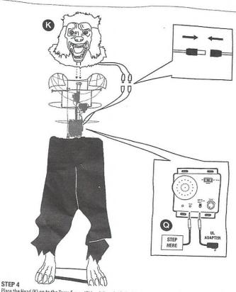
Place the Head (K) on to the Torso Frame (G) by sliding the forked-book into "neck" slot housing on the top of the Torso Frame (G), then connect the color coded male/female cable from the Head (K) to the Function Control Box as
