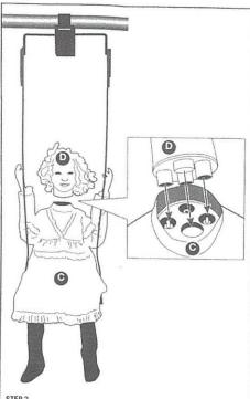
Firmly set the (D) Head on the neck of the doll on the (C) Mechanism with Doll as shown, making sure that the collar of the costume is not in the way of the
