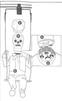
Firmly set the (D) Head on the neck of the doll on the (C) Mechanism with Doll as shown, making sure that the collar of the costume is not in the way of the assembly. Attach the (E) Hat to the (D) Head as shown.
