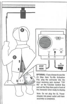
Find the Function Control Box located at the back of the (C) Mechanism with Doll, plug the UL Power Adapter into the input receiving jack marked "DC 5.9V" on the Function Control Box.
