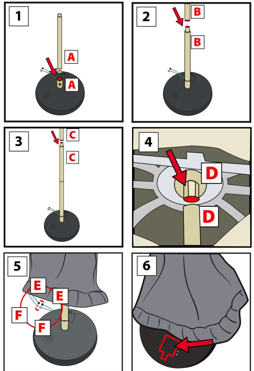
1. Insert BOTTOM POLE into the FLOATING BASE. (Match A to A) Pole is secure when snap lock pin clicks into post on base.
