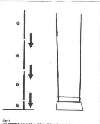
Now Assemble (B) Support Poles to (A) Base with the slot housings facing in as shown, and secure by aligning the quick-connect push buttons into the pre-drilled holes. Repeat this three times per side.
