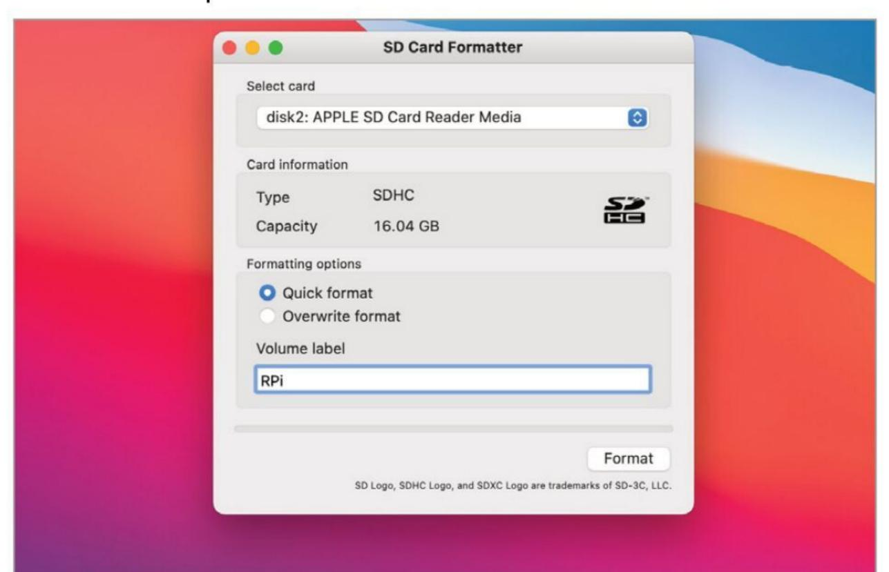
Make sure the card is present in the Select Card area; you should only have one SD Card inserted into your Mac. Open SDFormatter and choose the Overwrite Format option to ensure that all the old data is removed from the card. Enter a name for the card in the Name field to help you identify it; although this isn't necessary for the installation process.
