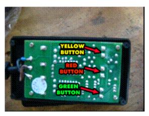
On the back of the circuit board opposite the buttons there will be two drops of solder for each button. We want the two that are for the **GREEN BUTTON**.
