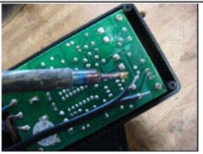
Solder each wire to the drops of solder for the **GREEN BUTTON**
