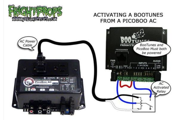
You must use a relay with 110v AC coil so that the PicoBoo AC can activate it.
