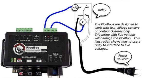
\* Any source that matches your relay. This could be AC, DC, 9v, 12v, 24v, 110v, 220v, etc.
