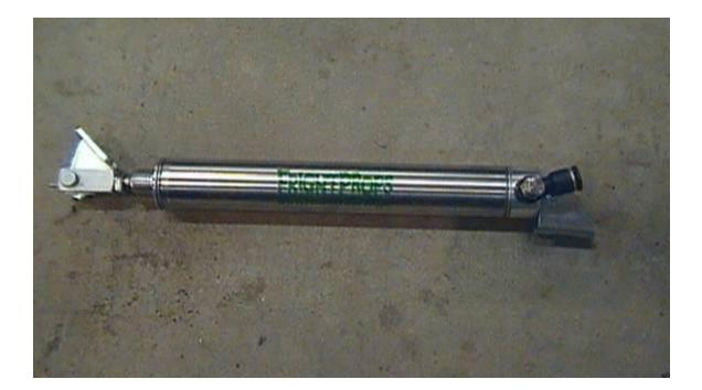
This is the base of your air cylinder. This picture is of the pivot bracket before it was welded on (yours will already be welded on, but it attaches the same way). This also shows a male connector with flow control (optional. The flow control will regulate how fast the cylinder retracts its rod). You can use any regular push-on male connector. Be sure to use pipe thread sealant tape when installing air hose pieces, and use a wrench to tighten.
