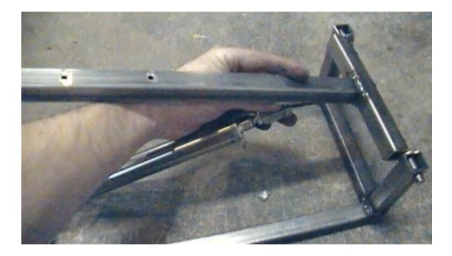
Be careful of mounting the clevis bracket too close to the arm's pivot point. If you do, the arm will want to swing down instead of up, and the rig will lock up.
