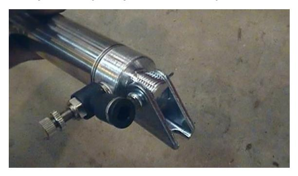
Below is the "nose" of the cylinder with a clevis and clevis and clevis mounting bracket installed. You may need a washer to take up the extra length of the pin holding the bracket to the clevis, to keep it from wobbling.
