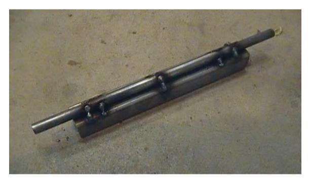
Take your left over, extra long piece of 3/4inch square tubing and cut it to whatever length you want the arm of your flipper rig to be (length in the photo is 18inches). Go ahead and drill some holes in it. These will be the holes you will attach your prop or pieces of wood to.
