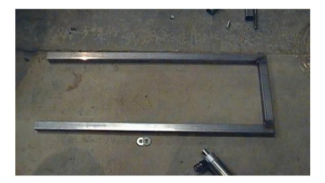
When you've completed this, feel free to drill a few holes in it. You'll be mounting this to a base of wood later. Just don't place holes too close to the bottom corners of the U.
