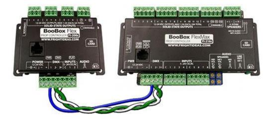
These are instructions on how to link slave BooBoxes to a master in Director. This will allow you to program as if they are all one controller. You first need to link them together by wiring their DMX pins 1,2, and 3 together as shown in the diagram. It is important to use twisted pair for pins 2 and 3 (see BooBox manual for more info on that).
