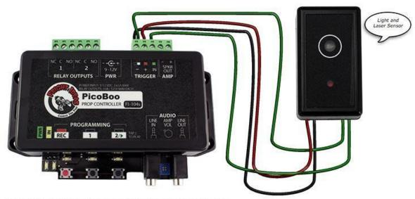
Note: You must switch the trigger input of the PicoBoo to accept Normally Closed trigger input to use this sensor.
