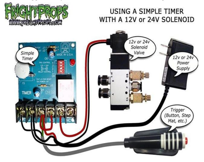
When using the FrightProps PIR the solenoid and power supply must both be 12V DC
