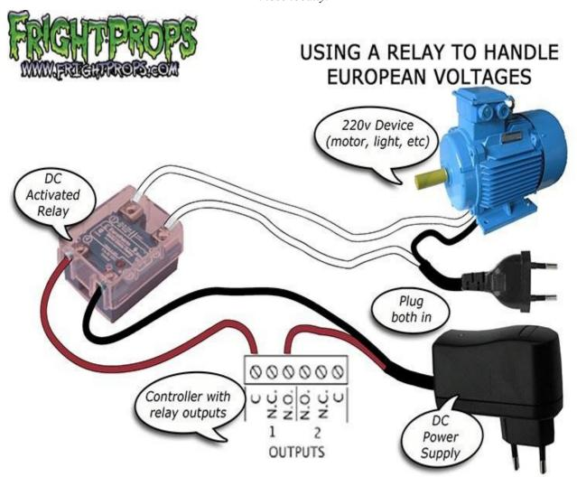
Use a relay that can handle the VOLTAGE and AMPERAGE of the load that you will be using. It must also have a 12v DC coil that activates it. Note: The two POWER plugs should both be plugged in to an outlet or power strip at all times.
