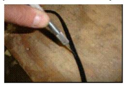
Use a sharp utility knife, x-cto knife, or scissors to separate the two wires on the AC cable of your device.
