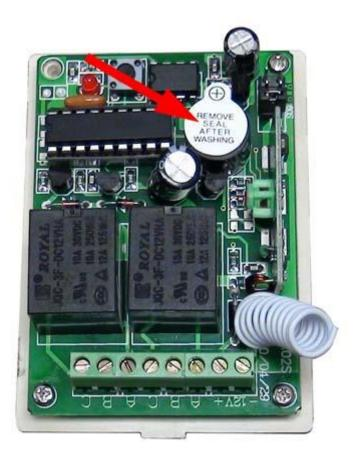
If you have a soldering iron the best way to remove it is to de-solder it from the circuit board.
